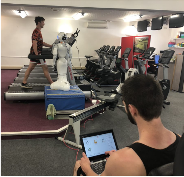
Fig. 1. Our C25K robot coach guiding a participant through an exercise session, supervised by the fitness instructor who can initiate robot actions, and respond to actions suggested by the machine learning system, through the teaching interface.
