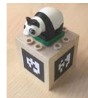
Figure 2. Object with a fiducial marker, which allows it to be identified and tracked.
